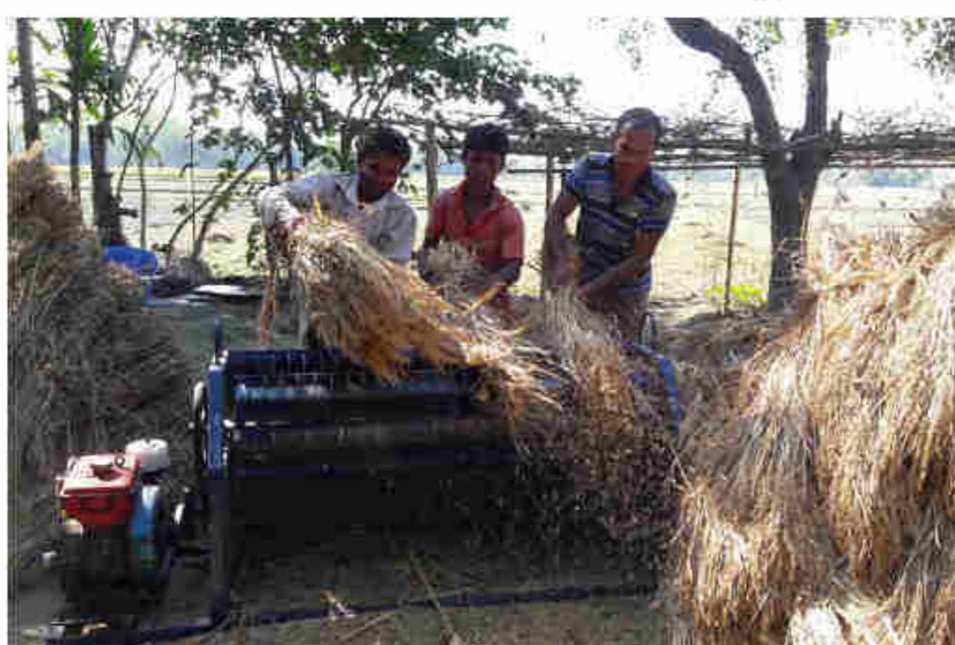
e. Mechanical threshing
