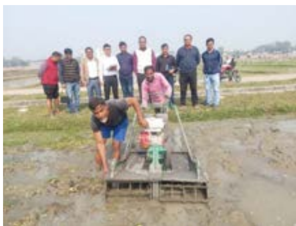
Plate 9. Test of modified hydro-tiller at BRRRI west byde, Gazipur.
