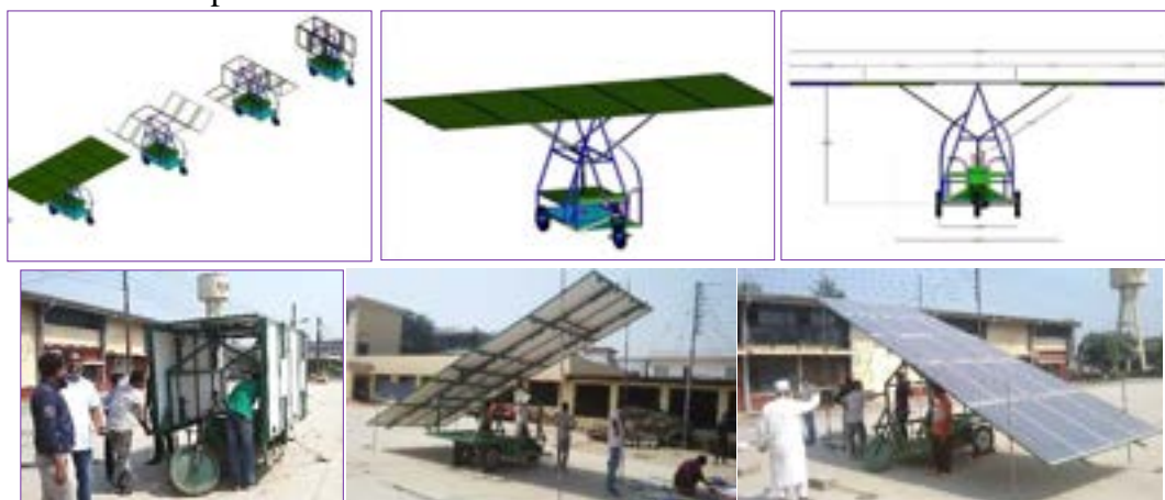
Figure 67. Solar panel array (arrangement) model 1(Previously designed)
