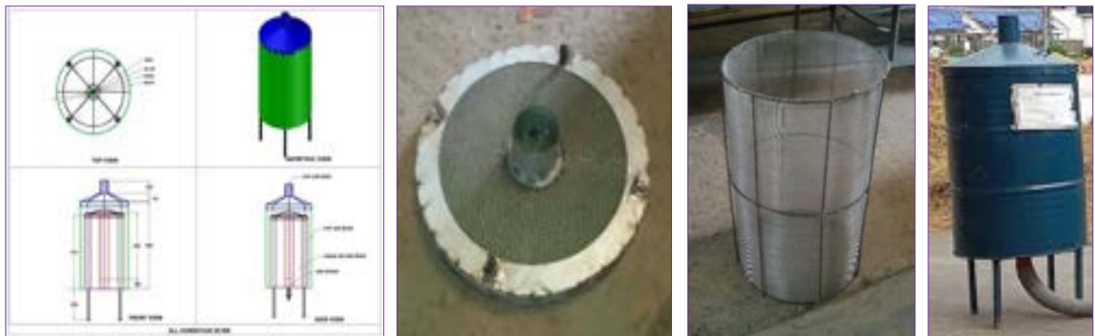
Figure 58. Drying chamber of the dryer.
