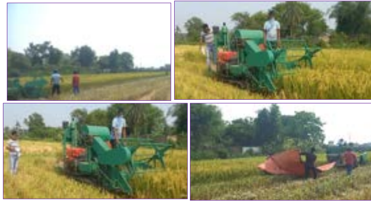
Plate 6. Performance test of the developed whole feed combine harvester.
