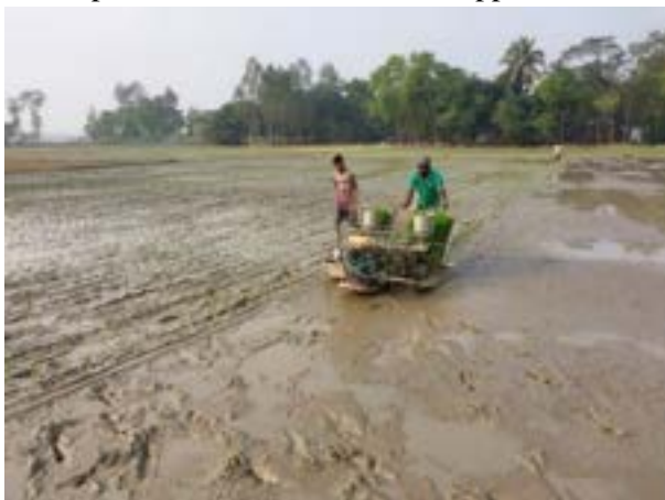
Plate 8. BRRRI developed rice transplanter cum mixed fertilizer applicator.
