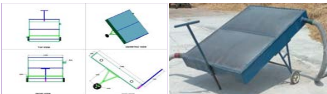
Figure 57. Solar collector of the dryer.
