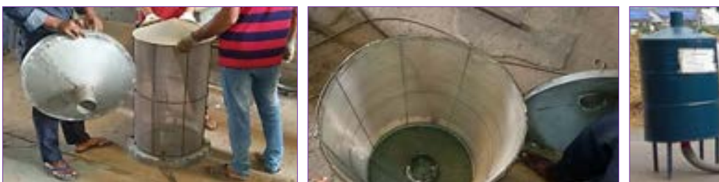
Plate 15. Photographic views of the perforated cylinder of the drying chamber.
