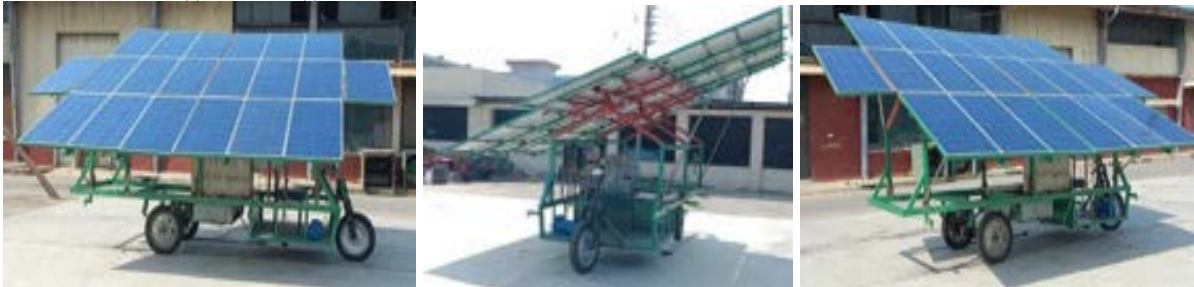
Plate 18. Solar-powered self-propelled mobile solar panel carrier
