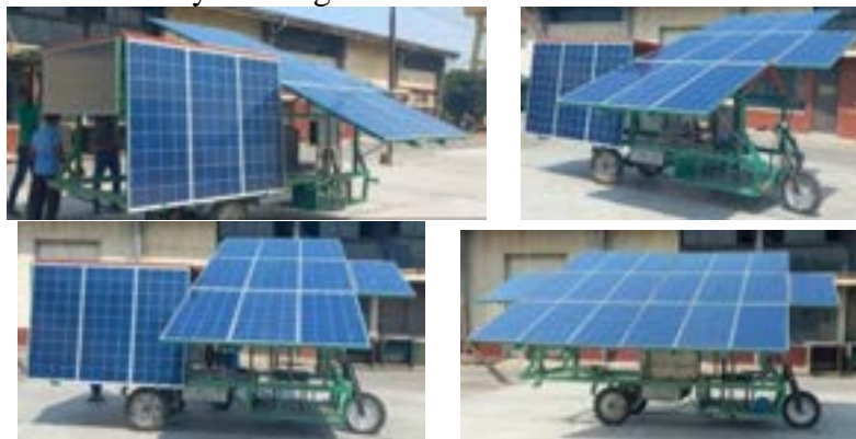
Plate 24. Adjustable panel angle with the carrier
