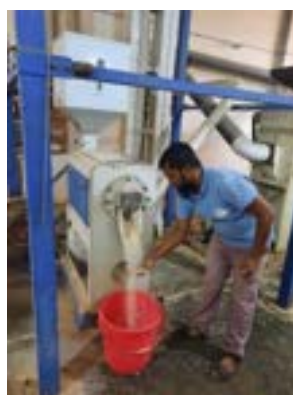
Plate 14. MNMP-15 friction type polisher in operation
