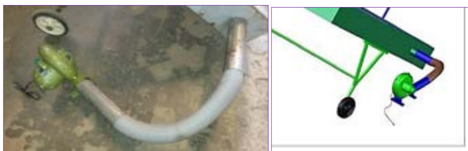
Figure 59. Blower of the dryer.
